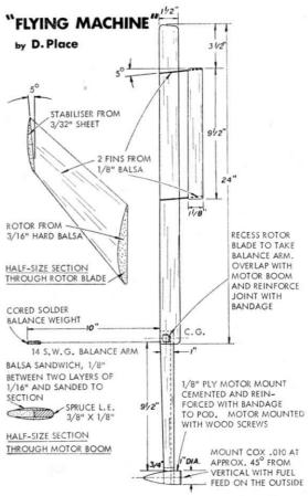
POD BUILT UP FROM TWO LAMINATIONS OF 1/2" BALSA
