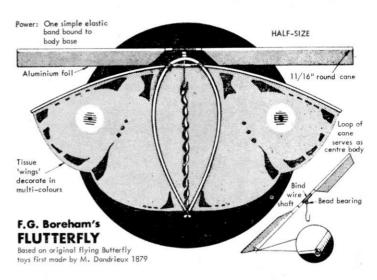
Flutterfly is very simple. Start by bending 72 x 1/16 in. cane to shape of body join by binding at the base. Wing spar is 7 in. of cane bound in position as shown. Drill or make a hole through the cane for the propeller shaft wire to work freely. The propeller is made with a 7 in. cane spar and blades of aluminium paper glued as shown, don't forget a spot of oil on the shaft for best results and climb!
